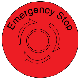
Figure 20. Emergency Stop Switch
